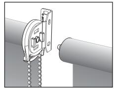
**Note:** If sharing a bracket between two shades, bracket can only be shared by a clutch and a pin end, not a clutch-to-clutch or pin end to pin end.
