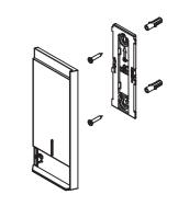
Use supplied fasteners and anchors to attach the base to wall.
