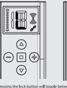
Pressing the lock button will toggle between locked and unlocked on LED screen.
