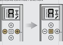
Select the desired Channel Double Tap the stop Button not the Level or Group you would like Control Bar, Now Press up or down to set the desired shade percentage. After 2 seconds the shade/s will move to that percentage.
