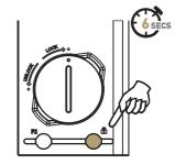
Repeat steps 1-6 for other motors. Once complete Press and hold the Lock button for 6 seconds while looking at the LED, and hold until L displayed.
