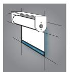
With a slight pull on the hem bar, the Semi-Auto cordless spring roller shade will automatically retract at a steady speed to a predetermined open position. Advanced updates to the traditional spring roller prevent over-cycling and unwinding at the top of the shade. You may also stop the shade band at any point as the shade is traversing up with another gentle pull of the hem bar.
